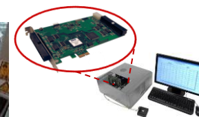
Network analyzer (measurement device for crystal oscillators)
